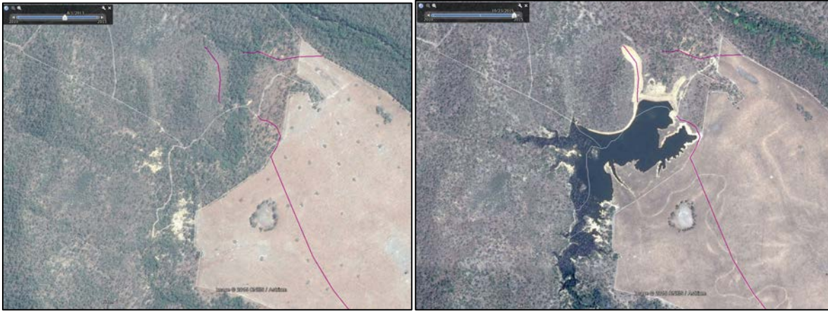
Figure 15 Default imagery shows a paddock with a variety of minor farm tracks in imagery dated 8/1/2013 (Cook paddock Springvale Station on the East Normanby River). Compared with more recent imagery from 10/23/2015 which shows a large farm dam has been built between the two time steps.
