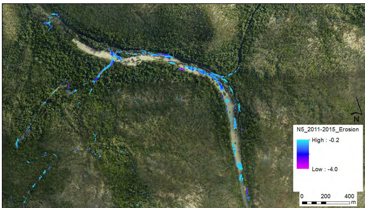
Figure A59: Erosion in main channel and secondary stream with orthophoto from 2009.
