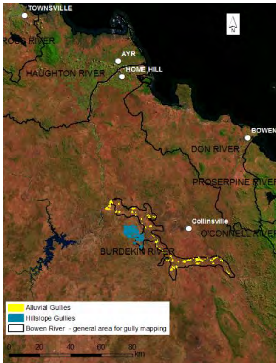
Figure 49: Map showing the area along the lower Bowen River within which there is a major concentration of largely highly active alluvial gully complexes. The areas mapped in blue are hillslope gullies in the Oakey Ck sub-catchment.
