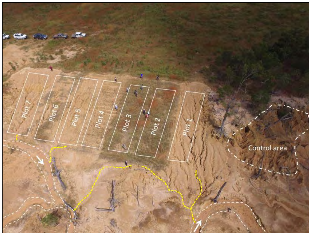
Figure 39: Oblique aerial photograph of the Crocodile trial plots with the control area (CRGC1-28) to the right (note the actual areas used for control erosion measurements are smaller plots within the area indicated. Note people/vehicles for scale (photo: John Brisbin).
